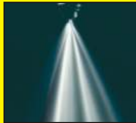
Clogged Fuel Injector
