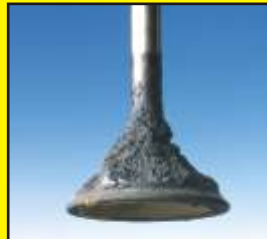
Dirty Intake Valve
